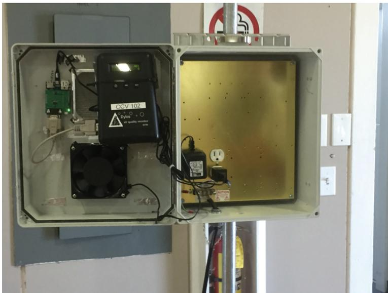
**Figure 1C:** A model of one of the Imperial County Community Air Monitoring Network's 40 air monitors. The weatherproof box is held off the ground by a stand made by the local high school's metal shop students, and contains a low-cost Dylos PM 2.5 sensor, a power source, and a small circuit board to transmit the data over WiFi.
